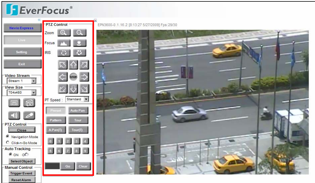
Figure 1-2 PTZ Control Window
